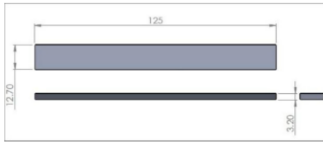
Figure 3-3 ASTM standard for flexural test (unit: mm). ( Kartikeyan B. et al.)
