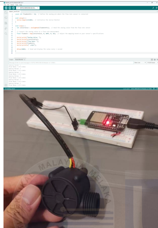
Water flow sensor testing
