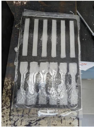
Figure 3.4.5.1: Samples after the hot compression molding process
