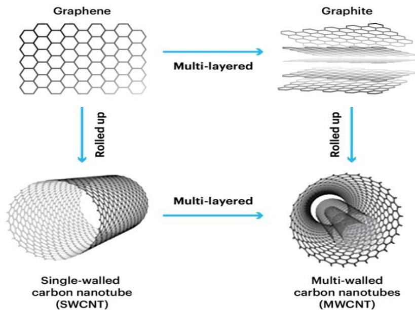
**Figure 2.2.2.1:**Schematic diagram types of carbon nanotubes
