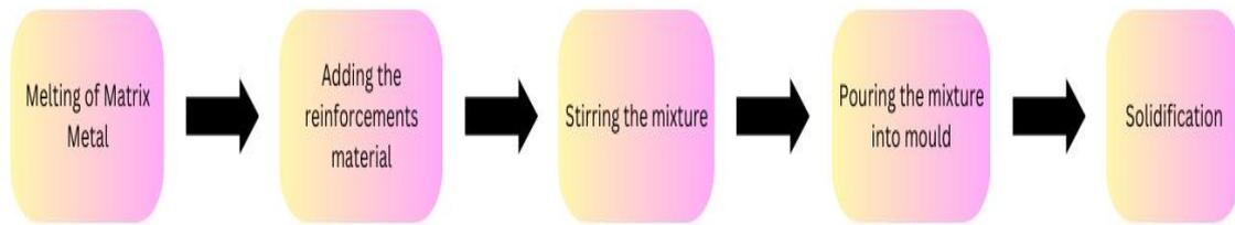
**Figure 3.6.1.1:** Permanent mould casting process flow
