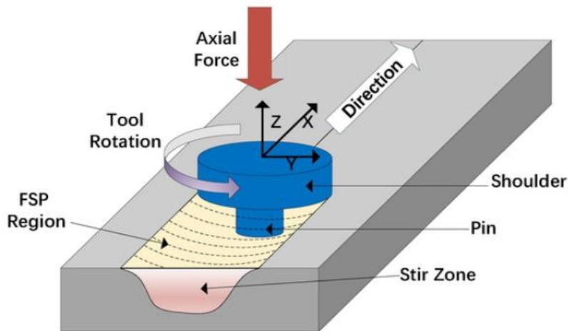
**Figure 2.5.4.1:** Schematic diagram FSP
