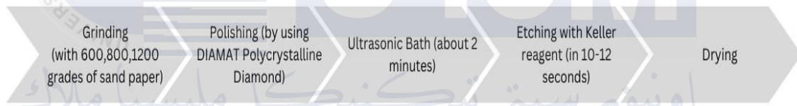
**Figure 3.7.3.1:** Flow of Sample Preparation
