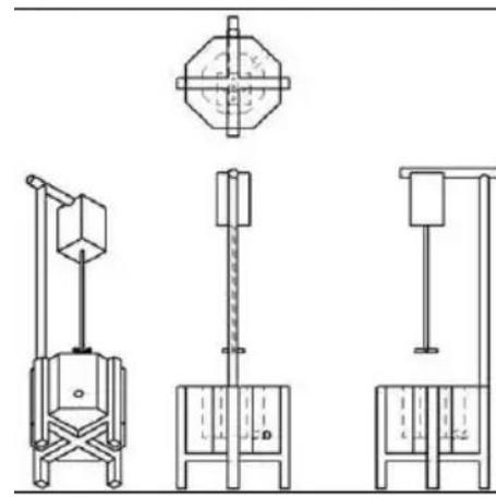
**Figure 2.4.4.2: Schematic Stir Casting**
