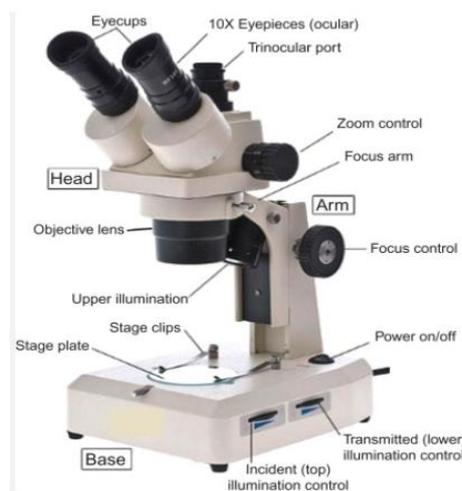
**Figure 2.6.2.1: Optical Microscope Parts**
