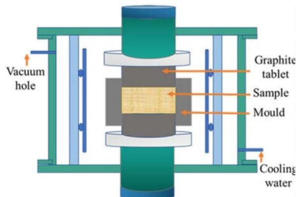
**Figure 2.5.1.2:** Ball Milling and Hot Press Sintering Diagram
