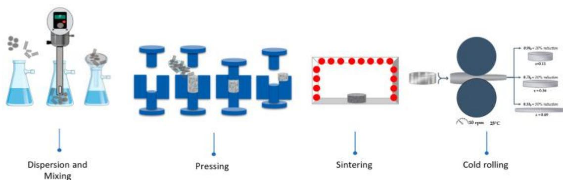
**Figure 2.5.1:** Powder Metallurgy Diagram
