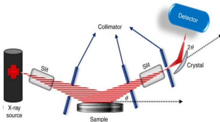
**Figure 2.6.1.2:** X-Ray Diffraction Diagram
