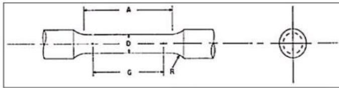
Figure 3.11 (ASTM E8M-04)
