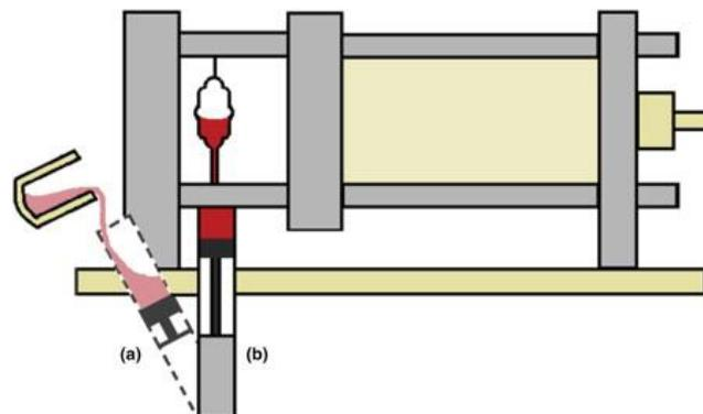
**Figure 2.4.2.1:** Indirect squeeze casting
