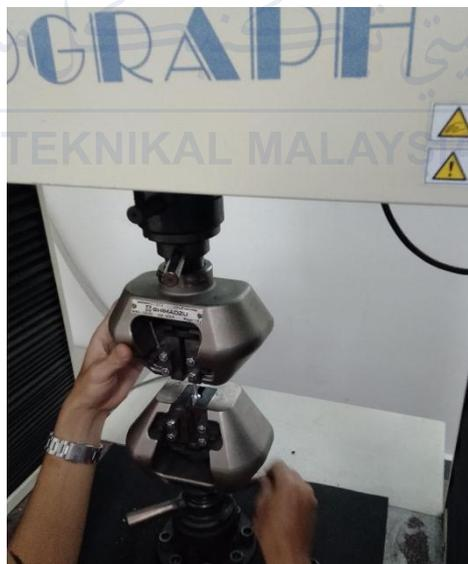
Figure 3.8.2: Tensile Test machine
