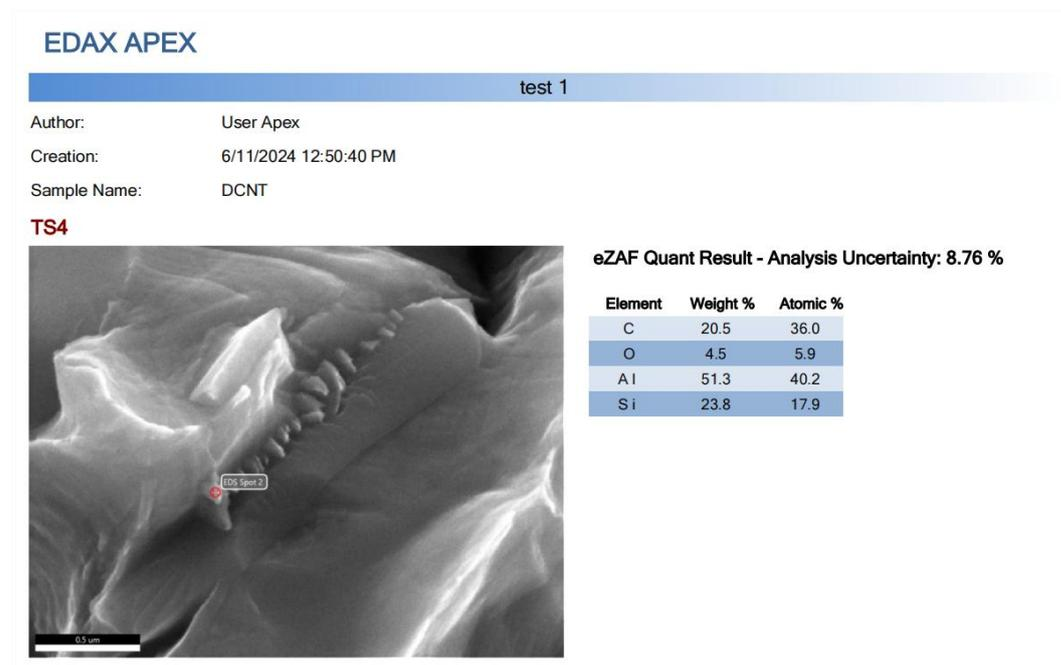
ii .Sample AL<sub>2</sub>O<sub>3</sub> 1 gram,CNT 0.3 gram; after undergo T6 heat treatment
