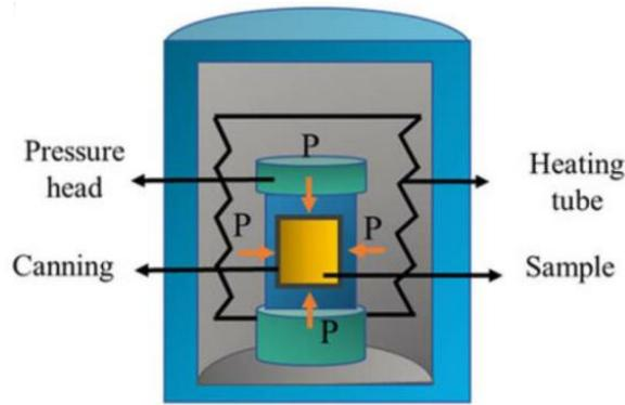
**Figure 2.5.2.1:** Hot Isostatic Pressing Process
