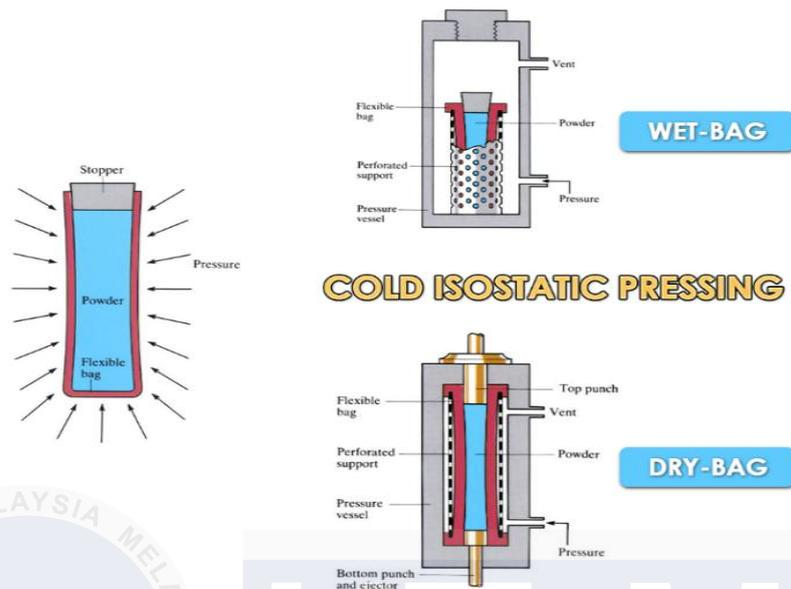
**Figure 2.5.3.1:** Cold Isostatic Pressing Diagram
