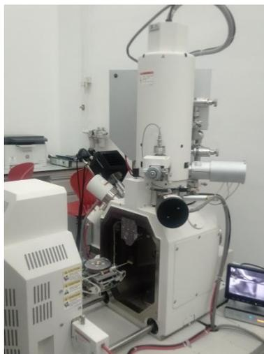
**Figure 3.7.3.2:** Model Evo, Hitachi FESEM machine
