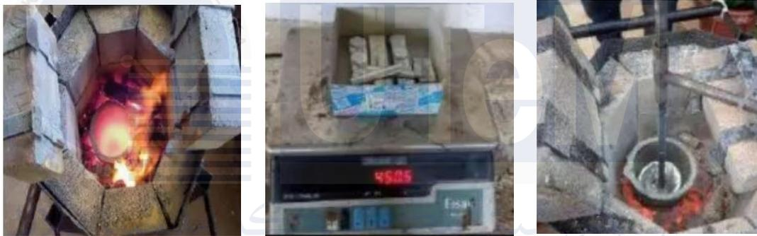
**Figure 2.4.4.3:** Heating furnace, cut into small pieces and stir molten metal
