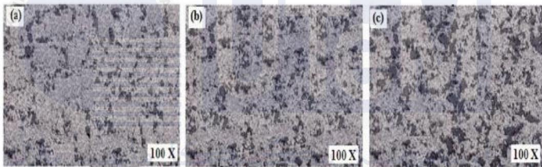
**Figure 2.4.5.1:** Microstructure of aluminium reinforced with (a) 5% (b) 10% and (c) 15% of CNT
