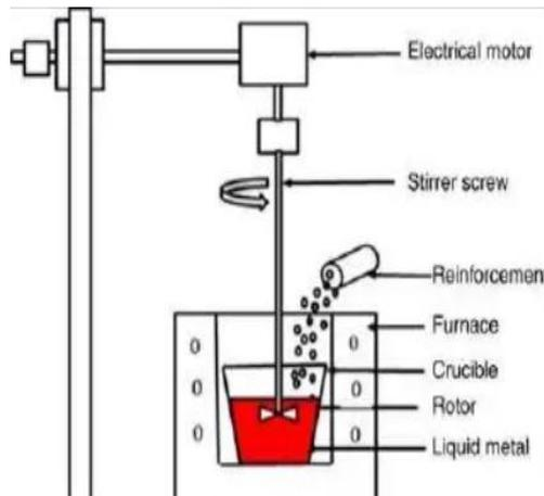
**Figure 2.4.4.1: Stir Casting**
