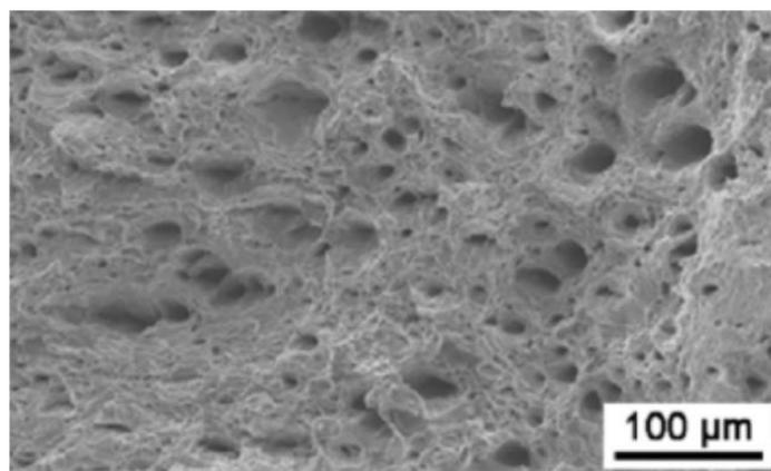
**Figure 4.4.1.1:** Dimple fracture obtained from the sample
