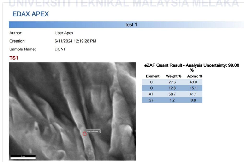
**Figure 4.3.6.2:** EDX results obtained for sample with CNT 0.8 gram
