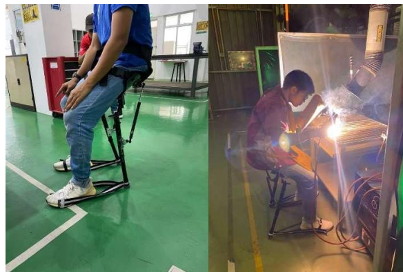
Figure 1.2 : Example of sit-stand exoskeleton design used in metal inert gas welding.
