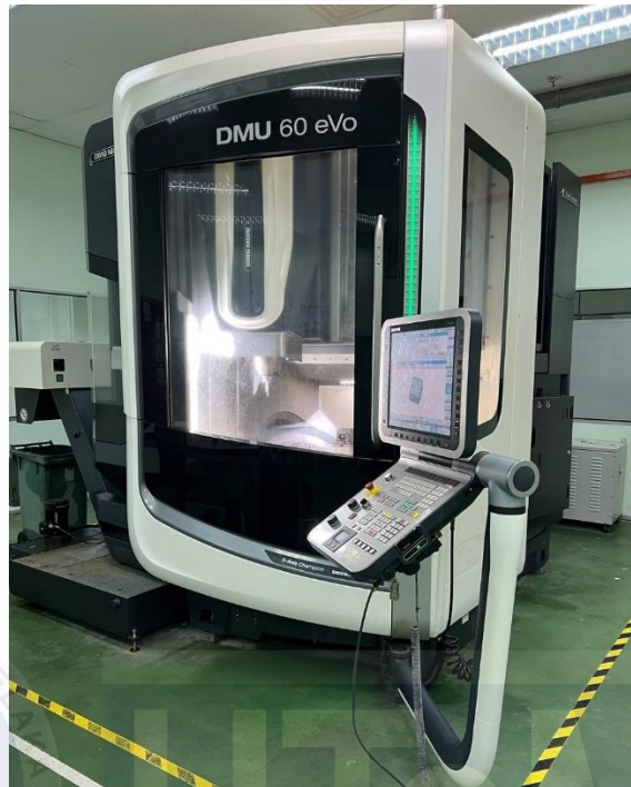
Figure 3.13 DMG MORI DMU 60 eVo CNC 5-Axis Milling Machine
