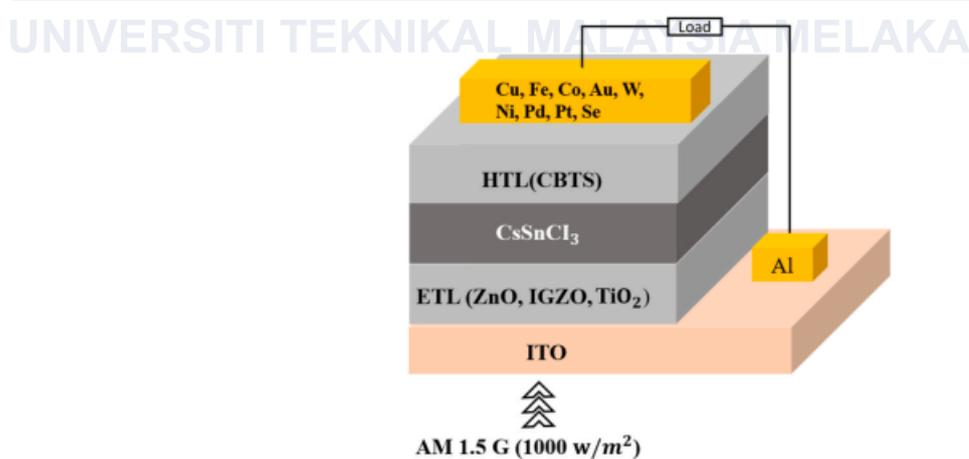
**Figure 2.5: Schematic diagram of the proposed perovskite device [11]**
