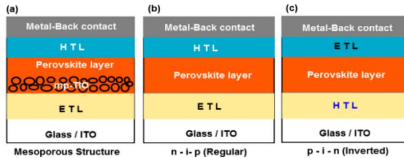
**Figure 2.1: Image of schematic illustrations for Perovskite Device Architecture [8]**
