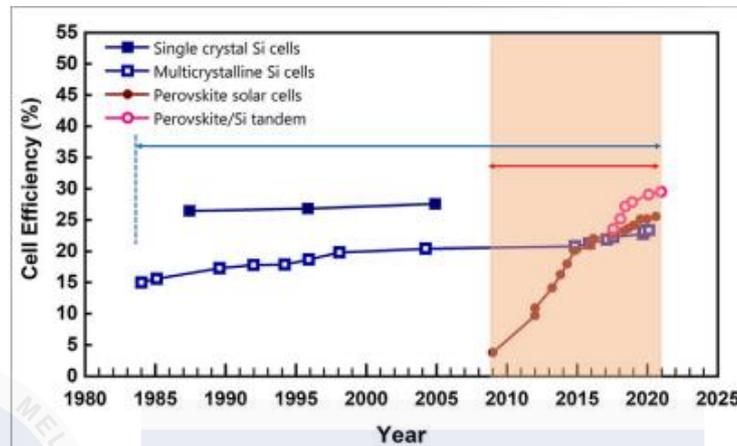
**Figure 2.3: Progress of cell efficiency in single crystal and multi-crystalline** [9]
