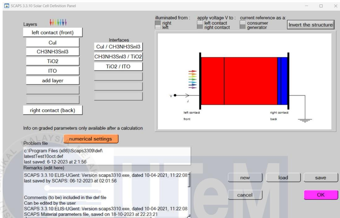
**Figure 3.4: PSC lead-free layers structure set-up**
