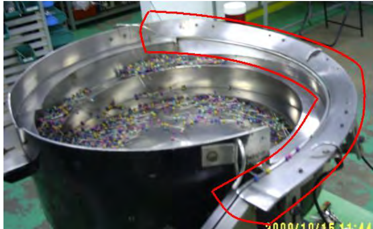
Figure 1.2: An illustration of bowl feeder, the region of the red line is the bowl feeder attachment, picture taken at Solid Heat (M) Sdn Bhd dated 15.10.2009
