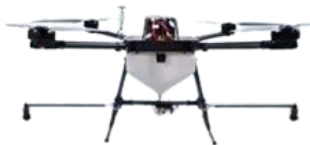
Figure 2.2 UAV used for spraying pesticide on crops [10]
