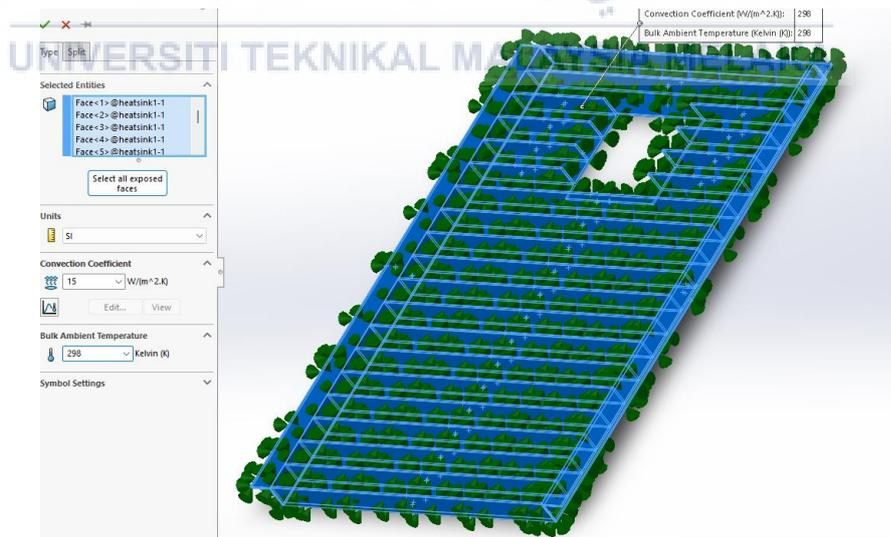
Figure 3.5.7 Convection characteristics (Front)
