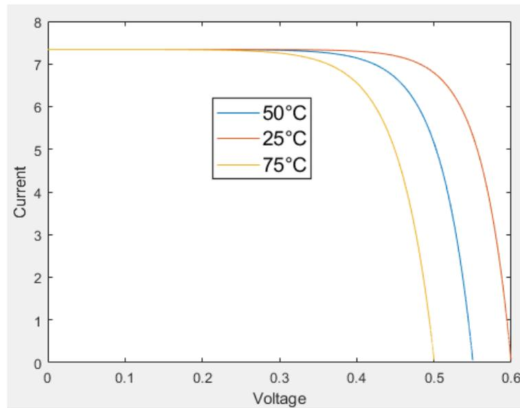
Figure 4.1.1.2 I-V curve for Temperature
