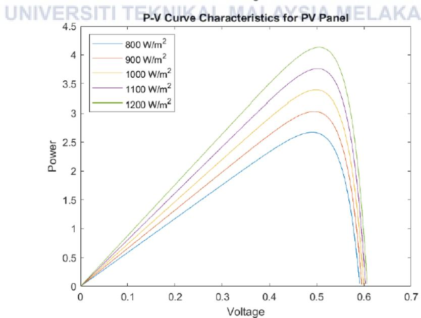
Figure 4.1.1.3 P-V curve for Power
