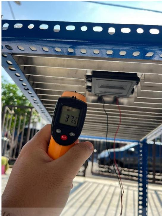
Figure 3.6.3 Temperature taken for solar panel with aluminium cooling fins at 9:00 A.M.
