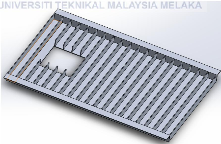
Figure 3.5.1 Overview of complete assembly of cooling fins
