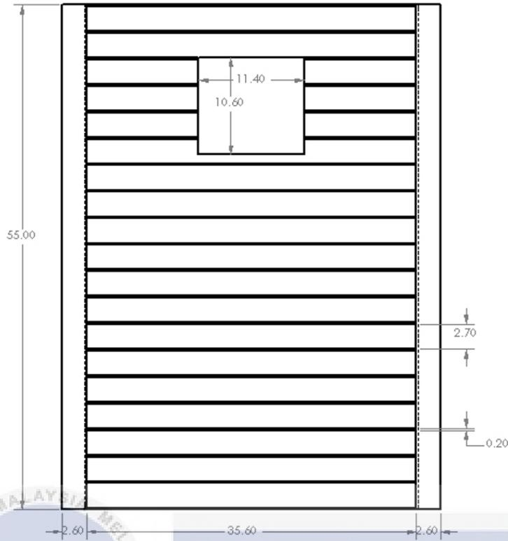
Figure 3.5.2 Dimension from top view
