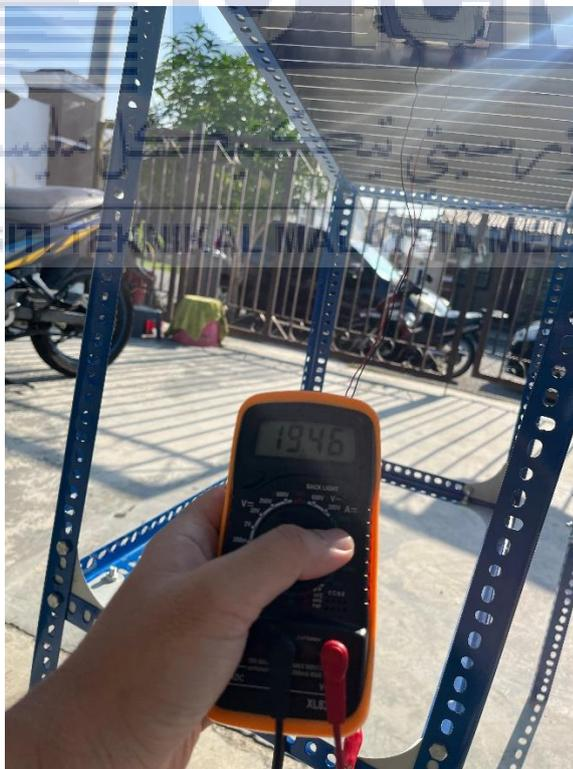
Figure 3.6.4 Output voltage taken for solar panel with aluminium cooling fins at 9:00 A.M.
