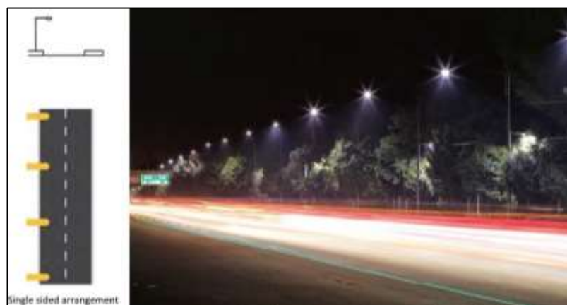
Figure 3.2 Single Lane Road with Lamp Pole on the Side
