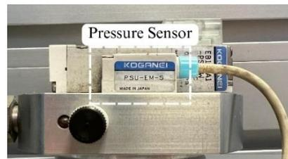
**Figure 3.4 Pressure sensor for IPA system**
