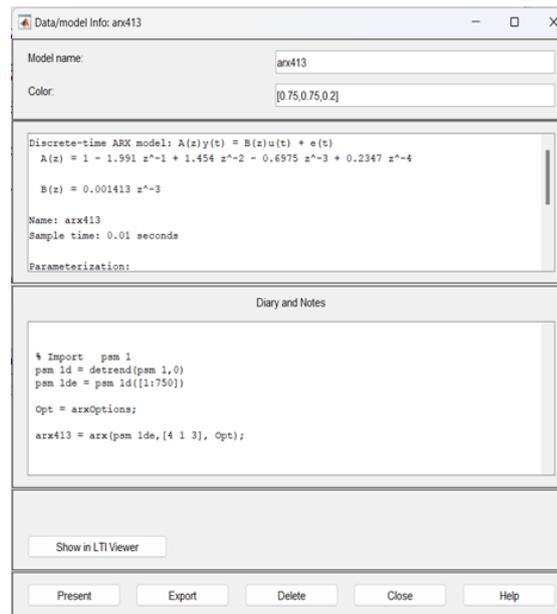
**Figure 3.17** The model info after the process of estimating
