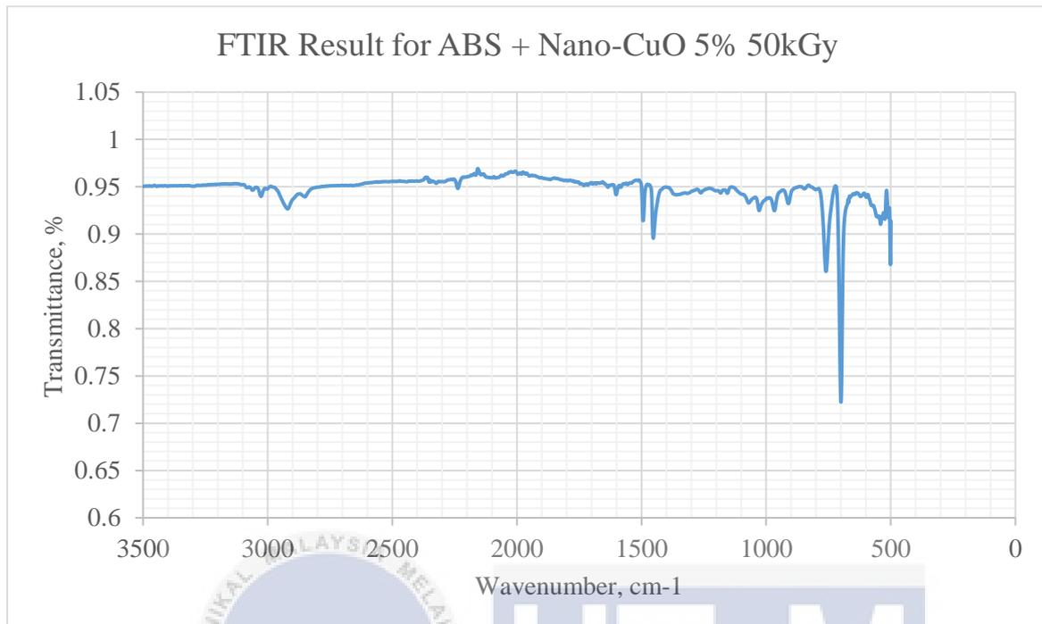
Figure 19: FTIR Result for 50kGy Radiated ABS+Nano-CuO 5%
