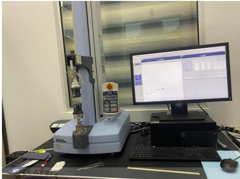
Figure 5: 1kN Tensile Test Machine.
