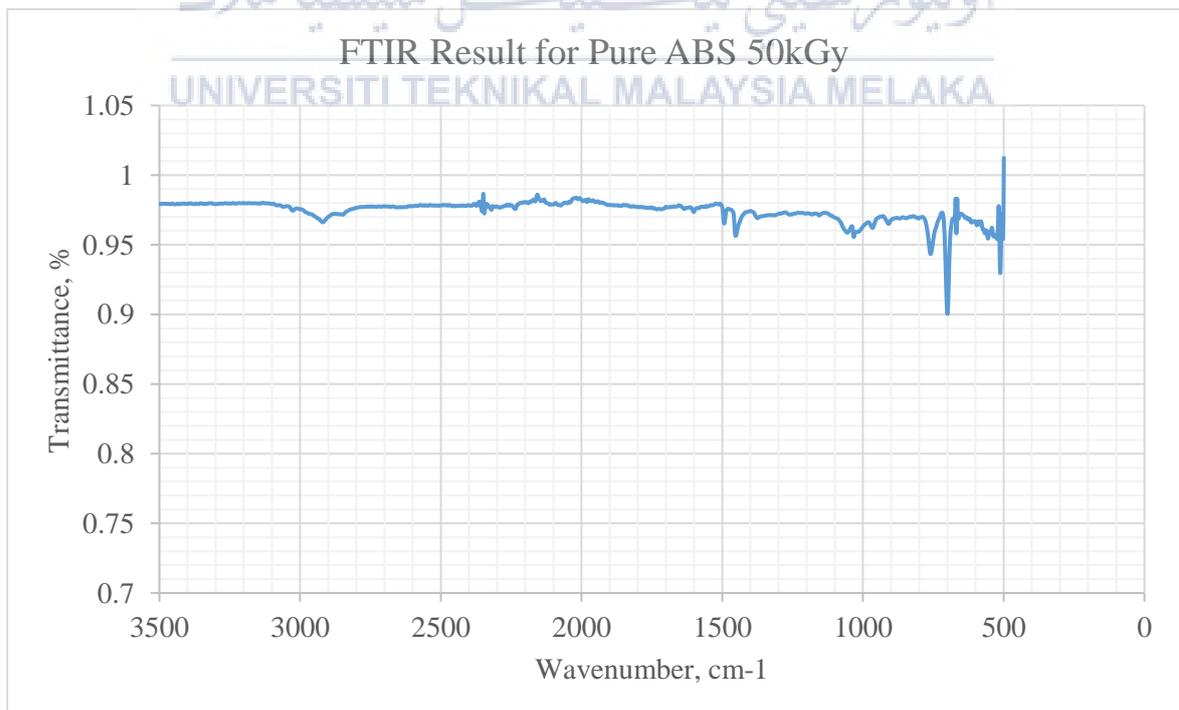
Figure 15: FTIR Result for 50kGy Radiated Pure ABS.
