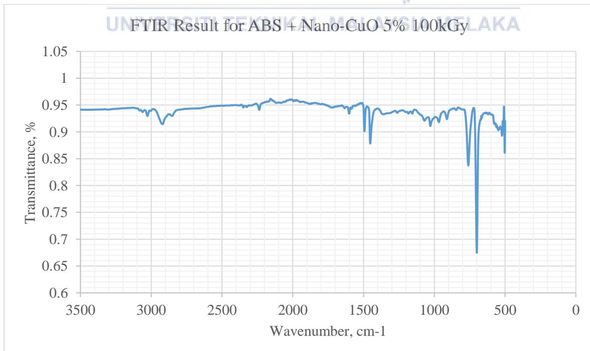
Figure 20: FTIR Result for 100kGy Radiated ABS+Nano-CuO 5%
