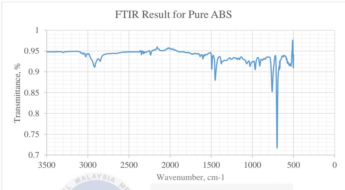
Figure 14: FTIR Result for Non-Radiated Pure ABS.
