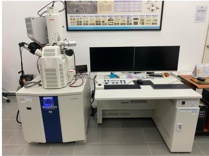
Figure 6: Scanning Electron Microscopy (SEM) and Energy-Dispersive X-ray Spectroscopy (EDX)
