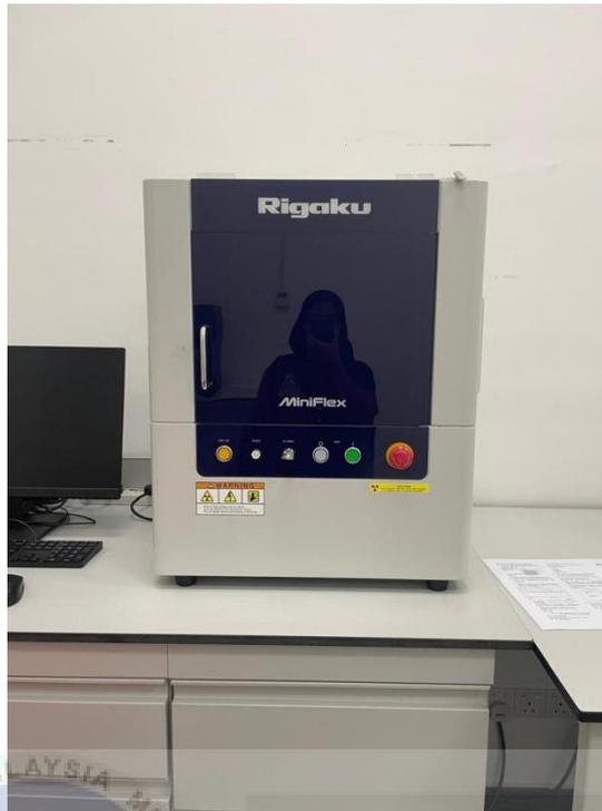
Figure 3.3 X-ray Diffractometer HyPix-400 MF
