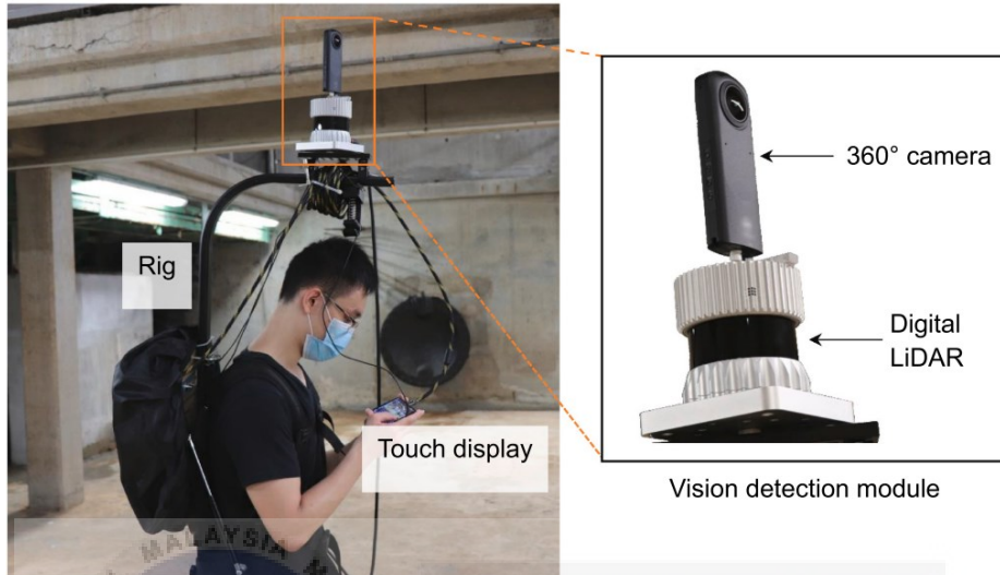
Figure 2.7: Automated defect inspection of concrete structure setup with 360° camera (Chow et al., 2021)
