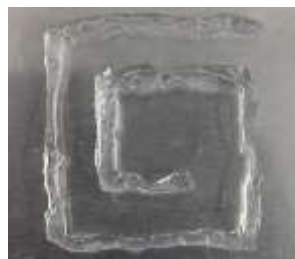
Figure 26: Sample print with optimized parameter
