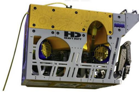
Figure 2.4: A Work Class ROV (WCROV) [13]
