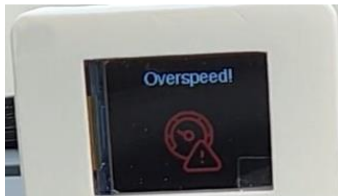
Figure 4-20 : Overspeeding shown on the TFT LCD of DMAS
