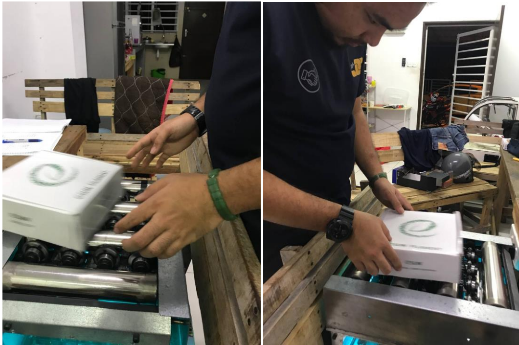
Figure 4.29: The omnidirectional Conveyor is in operation to place the load on the conveyor and test run.
