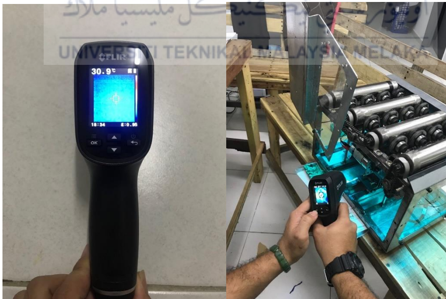
Figure 3.10: the digital meter temperature and example for check temperature at DC motor.
