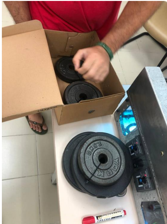
Figure 3.9: the sample dumbbell put it in the box for the load test at the Omnidirectional Conveyor product.
