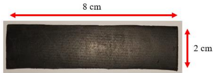
Figure 3.8 Size of NBR gasket
