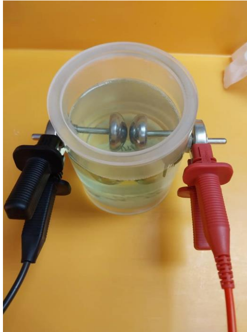
Figure 3.17 Chamber for PI testing
