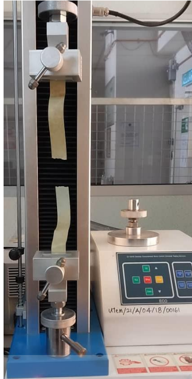
Figure 3.15 Torned TUK after tensile test
