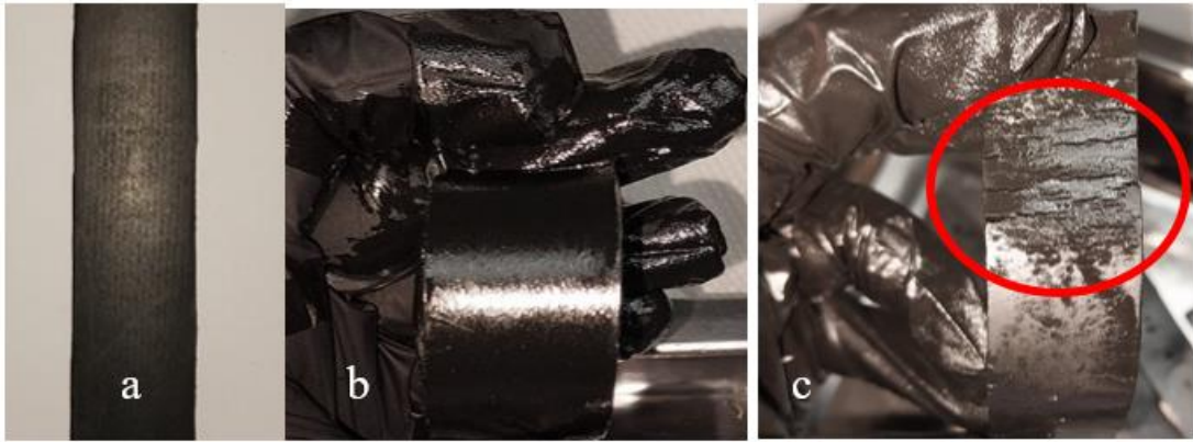
Figure 4.7 The surface of NBR gasket (a) initial condition (before ageing), (b) final condition in NEI (after ageing) and (c) final condition in SE (after ageing)
