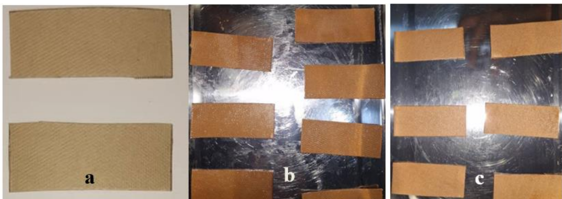
Figure 4.8 (a) Initial condition of pressboard (b) Final condition of pressboard immersed with TUK (c) Final condition of pressboard immersed with KP
