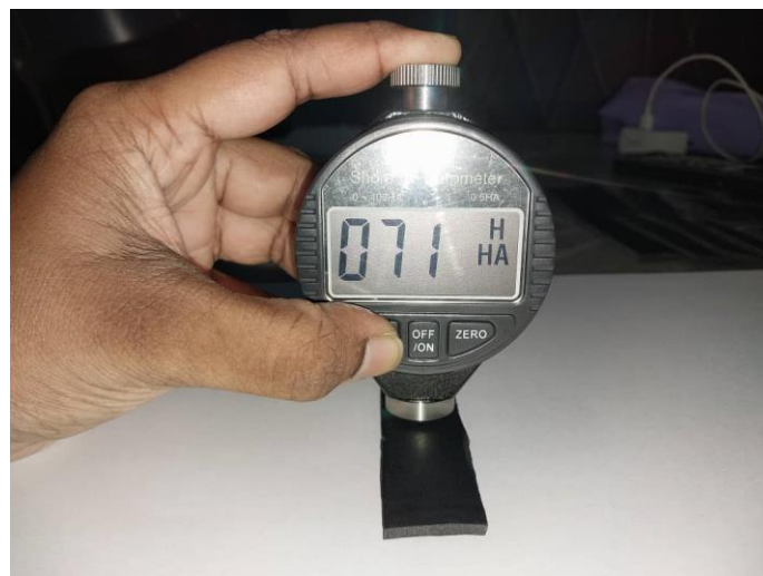
Figure 3.16 Measuring shore hardness of NBR gasket
