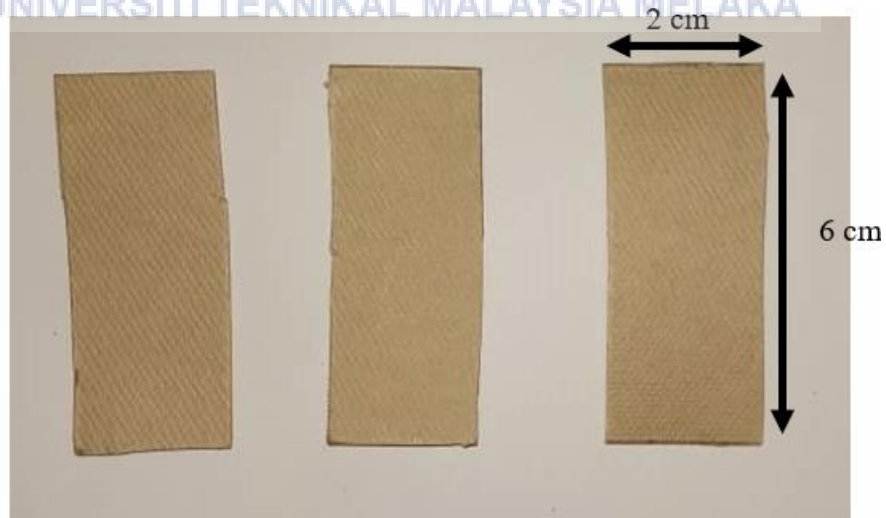
Figure 3.7 Size of pressboard
