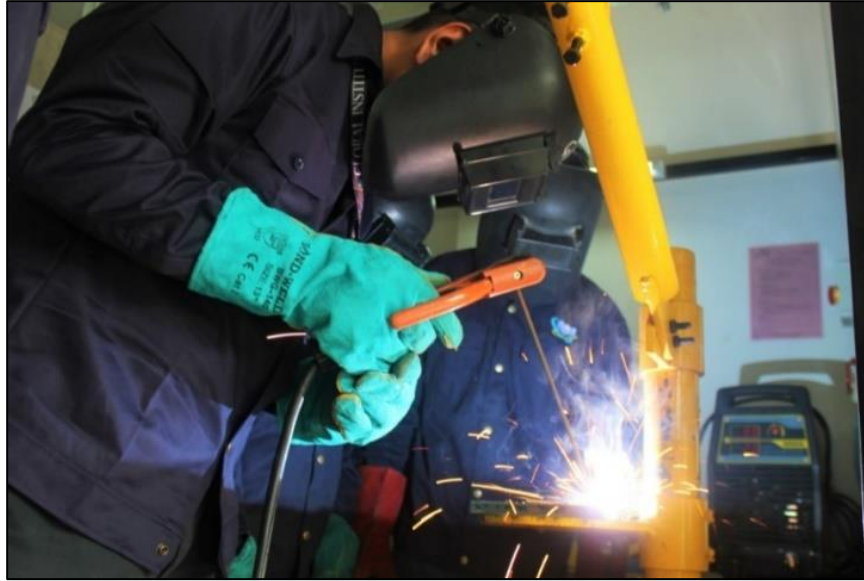
Figure 1.1: Shielded metal arc process (Global Institute of Studies, 2022)
