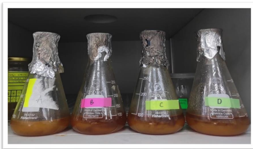
Figure 4.2: Samples of methyl ester from transesterification of different reaction temperature and reaction time.
