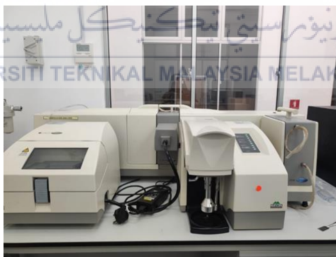
Figure 3.4: Particle Size Analyzer machine.
