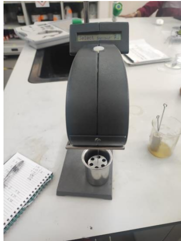
Figure 3.6: Viscotester 2 plus machine for viscosity testing.
