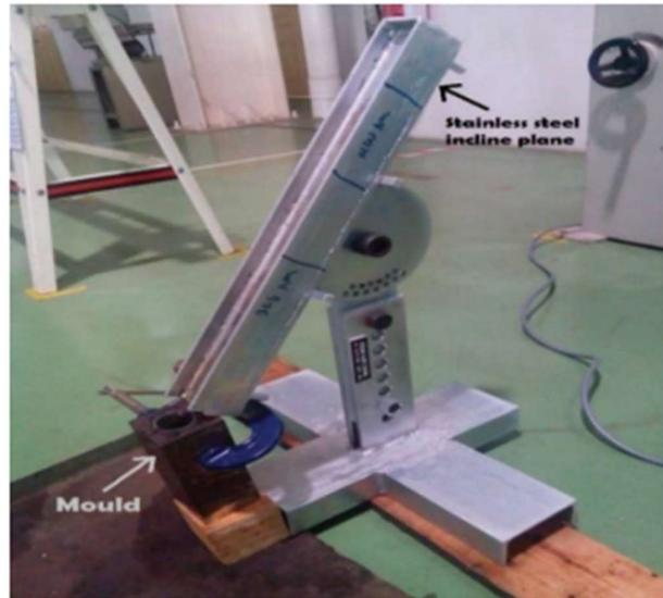
Figure 2-1 Cooling slope casting apparatus (Salleh et al., n.d.)
