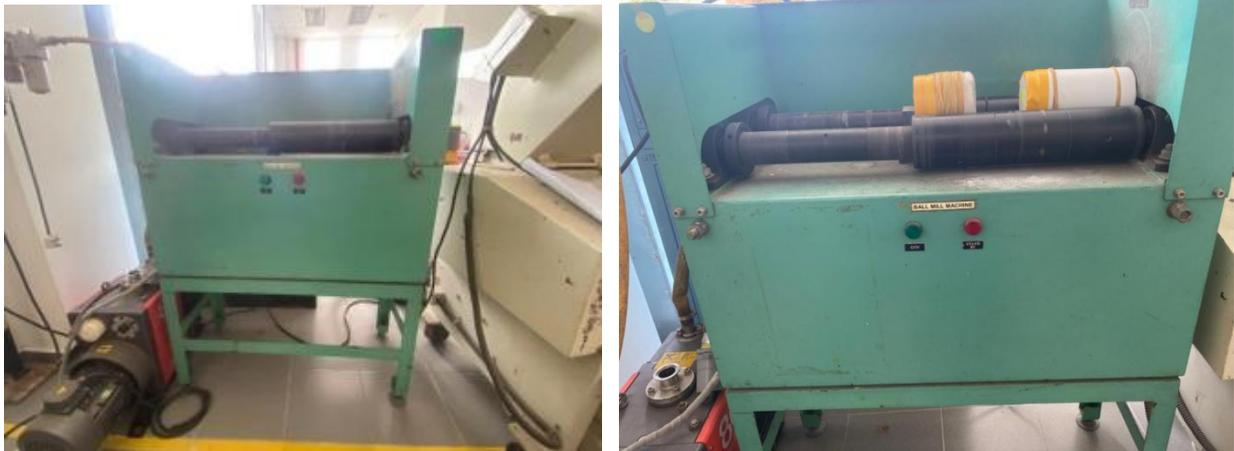
Figure 3.4.2: Ball Milling Machine
