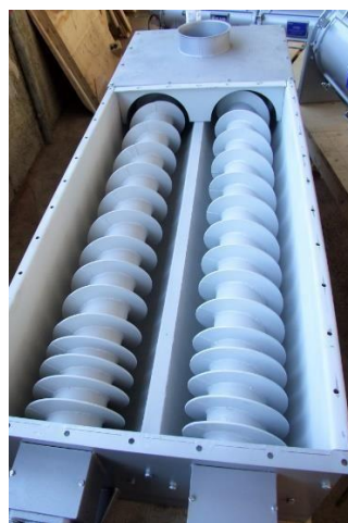
Figure 1.4 The worm conveyor (Source: Promid transportna tehnika, 2020)
