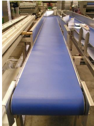
Figure 1.1 The belt conveyor (Source: H.S engineering Noido, 2017)
