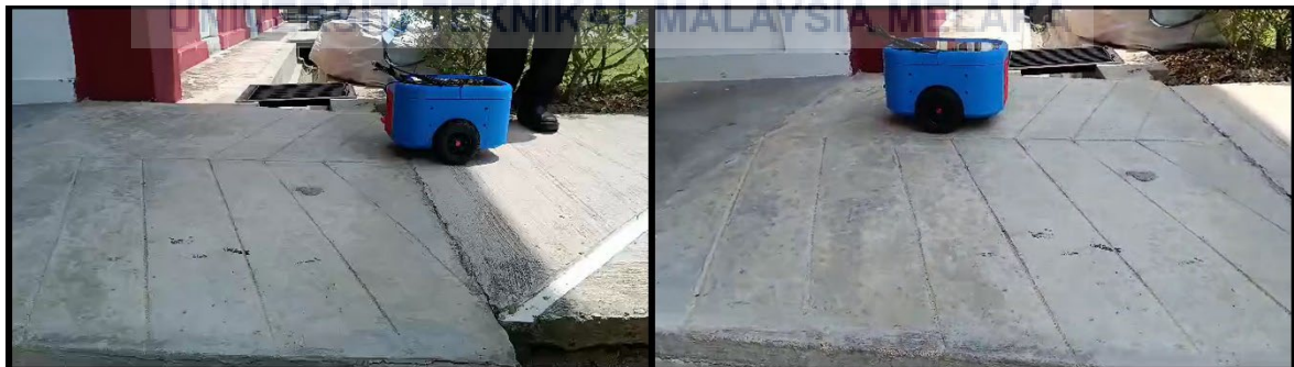
Figure 4.24: The differential drive mobile robot on a 5% slope in real-world conditions.
