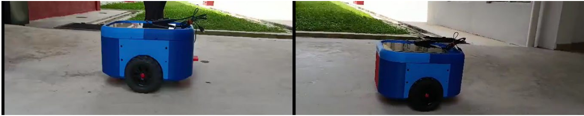
Figure 4.21: The differential drive mobile robot tested on a flat platform in real-world conditions.
