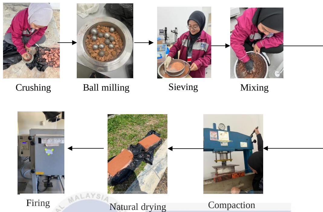
Figure 3.4 Eco-Brick Development Procedure
