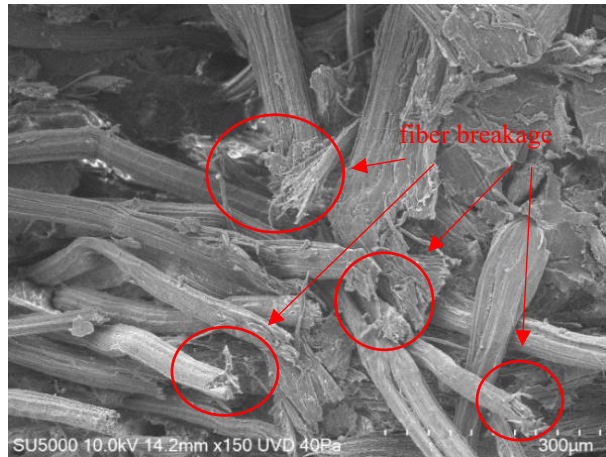
Figure 4. 11: SEM image of the fracture surfaces (30 wt% PALF fiber loading)
