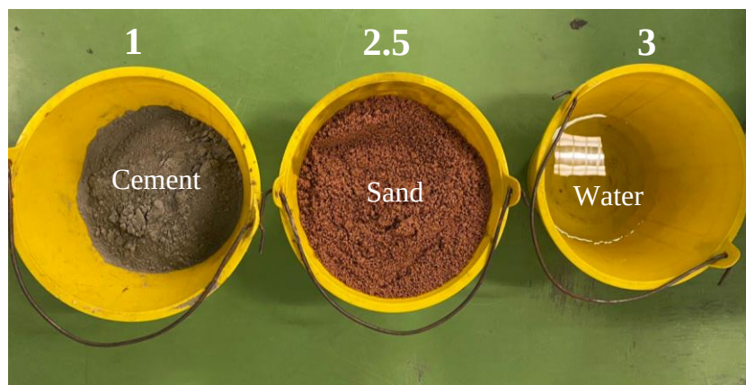
Figure 3.6: Concrete mix preparation
