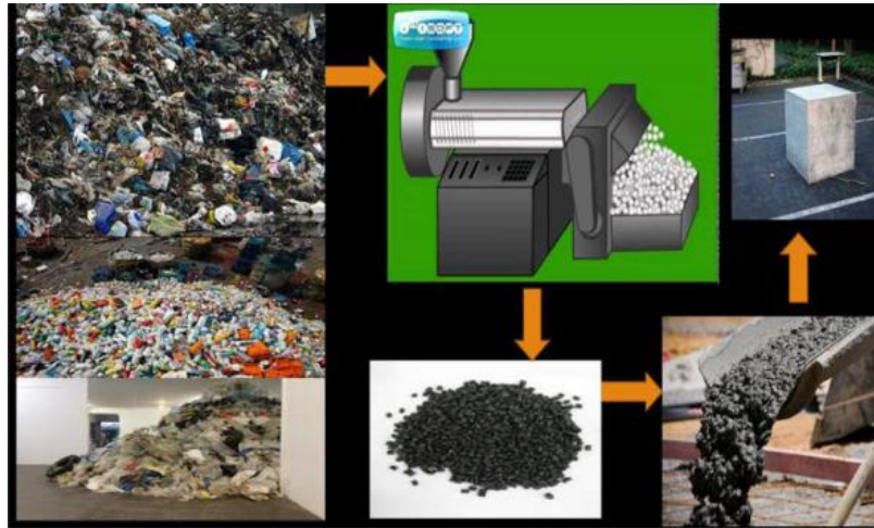
Figure 2.2: Plastic aggregate manufacturing process (Almohana et al., 2022).
