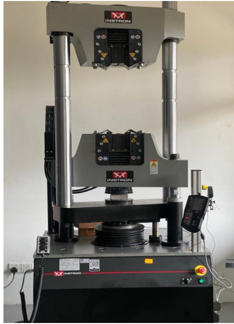
Figure 3.13: Universal Testing Machine Instron 600DX
