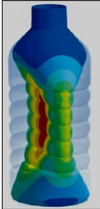
Figure 2.1: Buckling of plastic bottle (University of Alberta, ANSYS Advantages, 2008)
