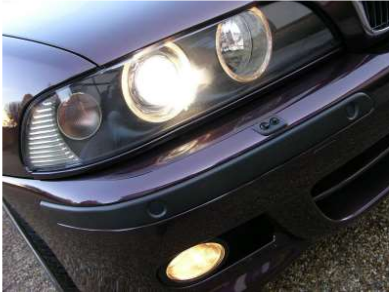
Figure 2.6 Halo Ring/Angle eye headlamp
