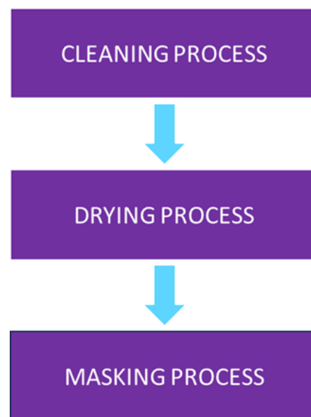
Figure 3.8 Thin cover glass substrate preparation process.
