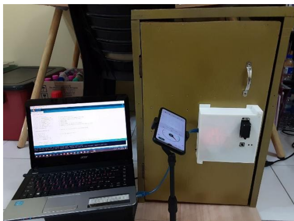
Figure 3.29 Position of measurement device at the door lock
