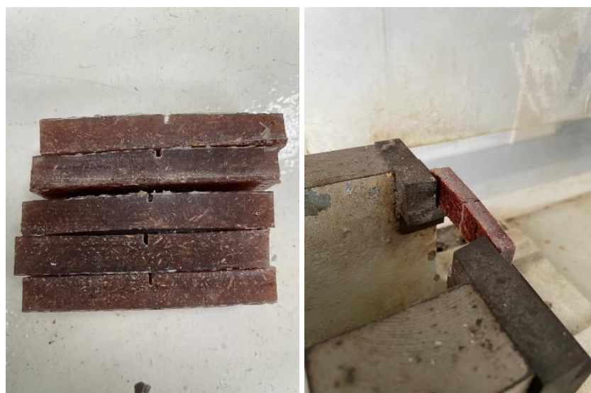
Figure 3.10 shows the process of impact testing.
