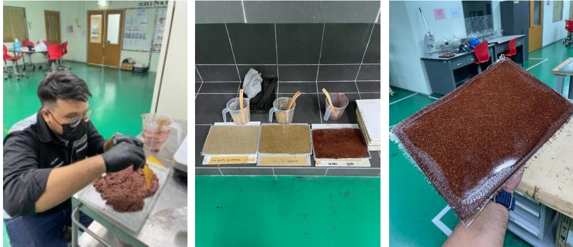
Figure 3.5 The fabrication and drying procedure
