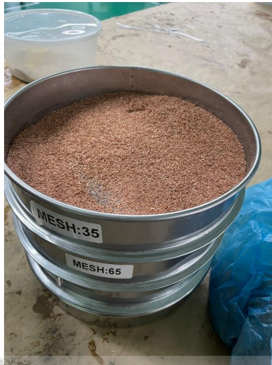
Figure 3.4 Mesh size of wood dust is at 35 mesh
