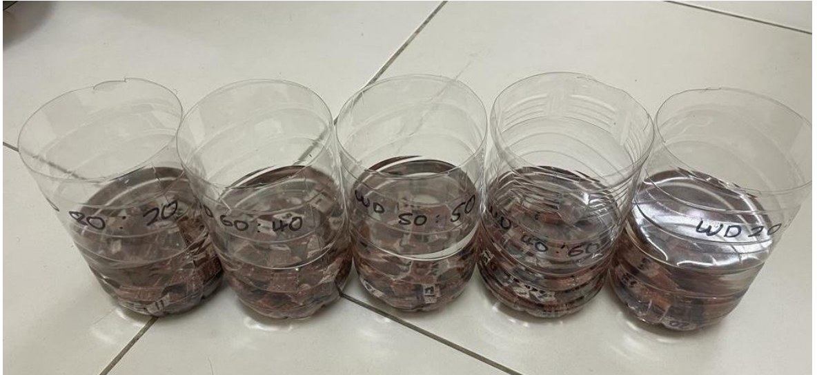
Figure 3.12 Shows the process of water absorption testing.
