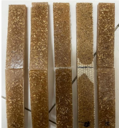
Figure 4.3 displays the specimen results after tensile testing that shows as the specimens are broken in half.
