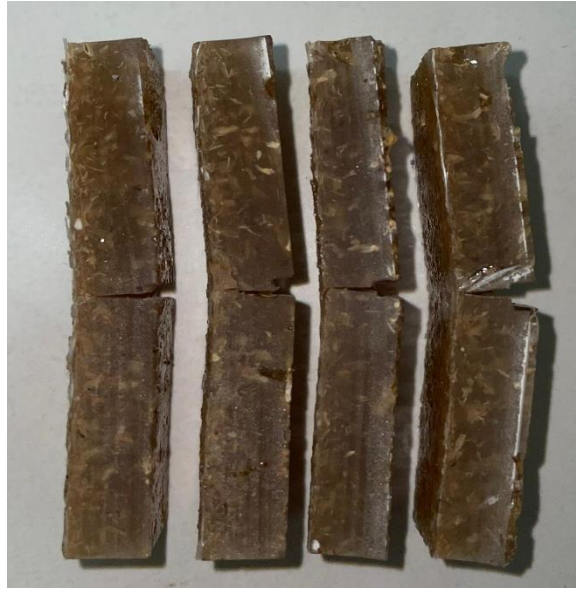
Figure 4.7 displays the specimen results after impact testing as the specimens are broken in half .
