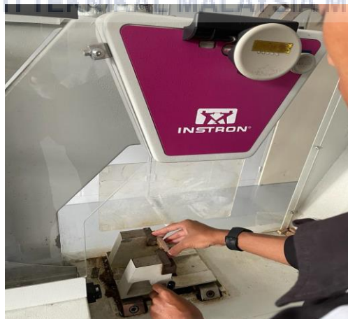
Figure 3.9 shows the specimen was tested using Instron Impact Machine to obtain results and followed by all ratios.
