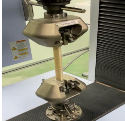
Figure 3.7 shows the specimen was being tested in tensile testing using universal testing machine and followed by all ratios to obtain results.
