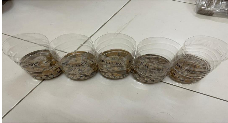
Figure 4.9 displays the immersion specimen during water absorption test for all ratios from day 1 until day 25.
