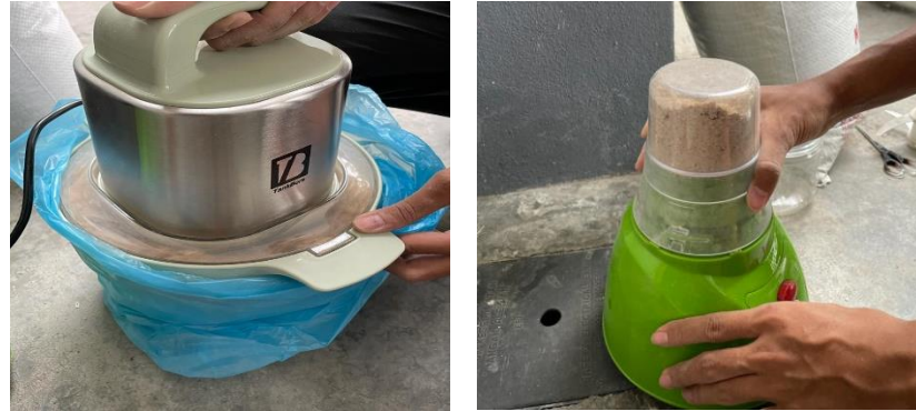
Figure 3.2 shows the raw rice husk was blended using blending machine to obtain rice husk ashes.
