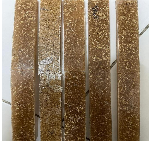
Figure 4.5 shows the specimen results after flexural testing as the specimens are broken in half.
