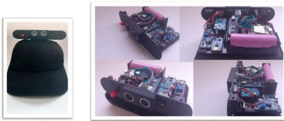
Figure 8: Internal structure of Smart Cap[6]
