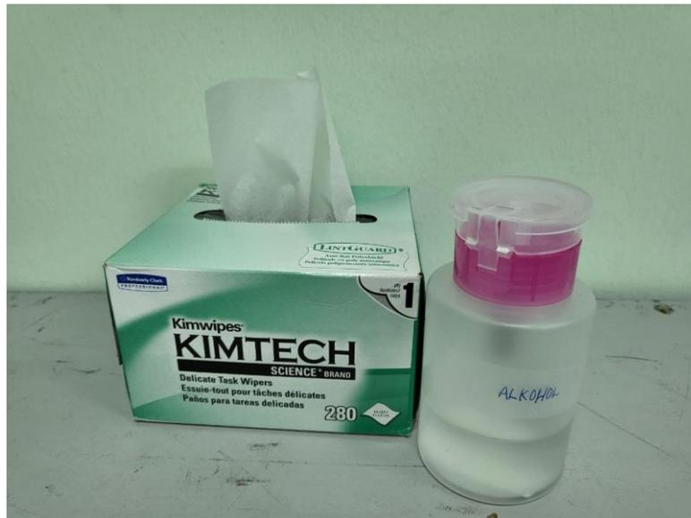
Figure 3.4: Cleaning tool used after stripping fibre optic cables
