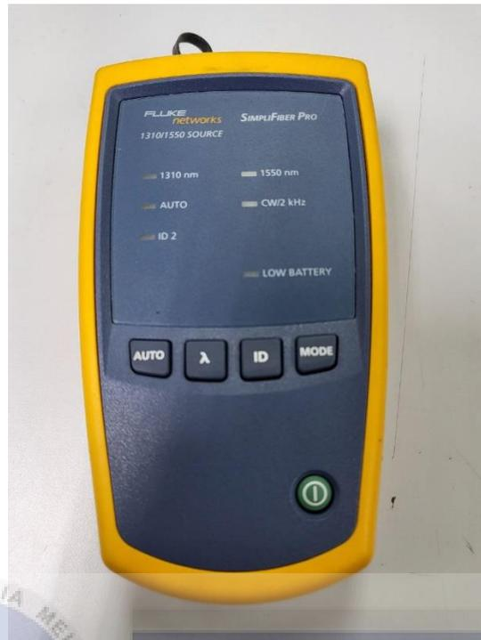
Figure 3.8: Light source that transmits wavelength of 1310nm and 1550nm light.
