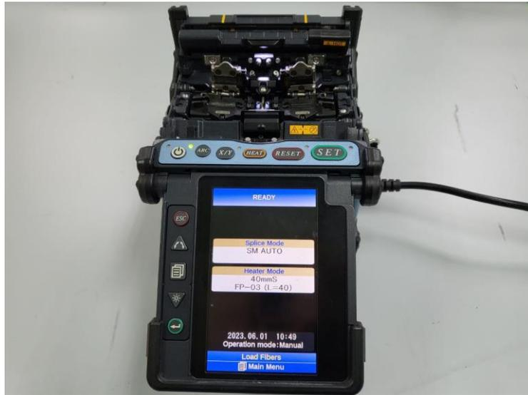
Figure 3.6: Fusion splicer machine which splits two fibres together automatically
