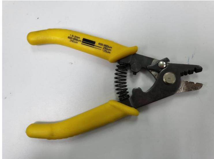
Figure 3.2: The Cutter to cut fibre optic cables
