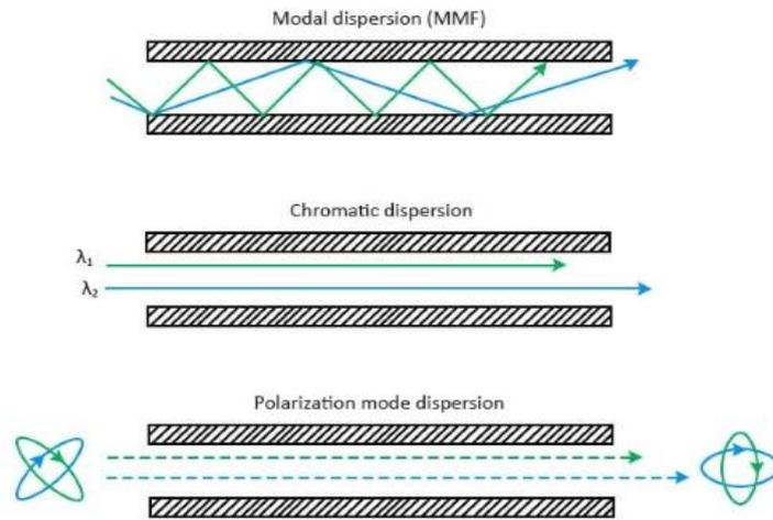
**Figure 3.26 : Three types of dispersion in fiber optics**
