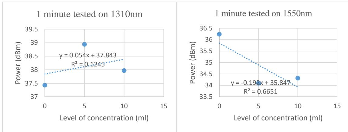
**Figure 4.8 : Microfiber Single Loop Sensor response at 1 minute**
