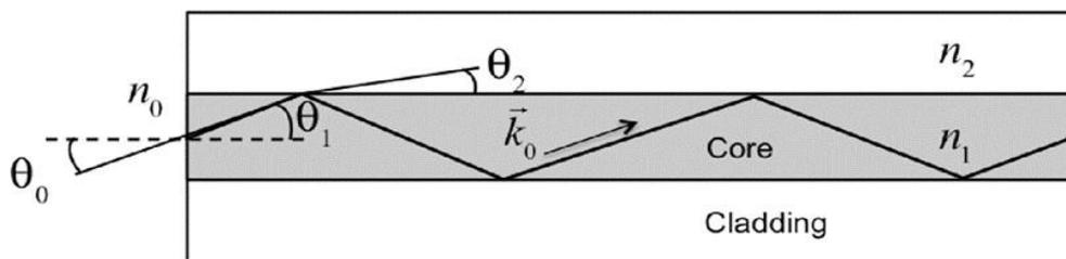
**Figure 2.8 : The way light enters and propagates through an optical fiber core**
