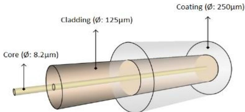
**Figure 2.2 : Structure of single-mode fiber**
