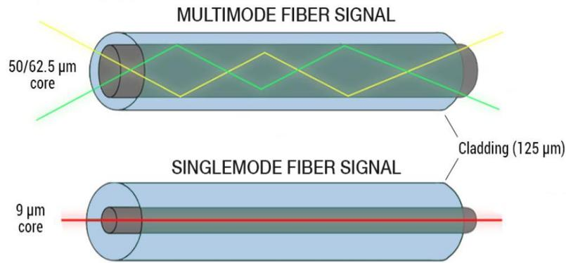
**Figure 2.4 : Difference between Mutimode and Single mode fiber**
