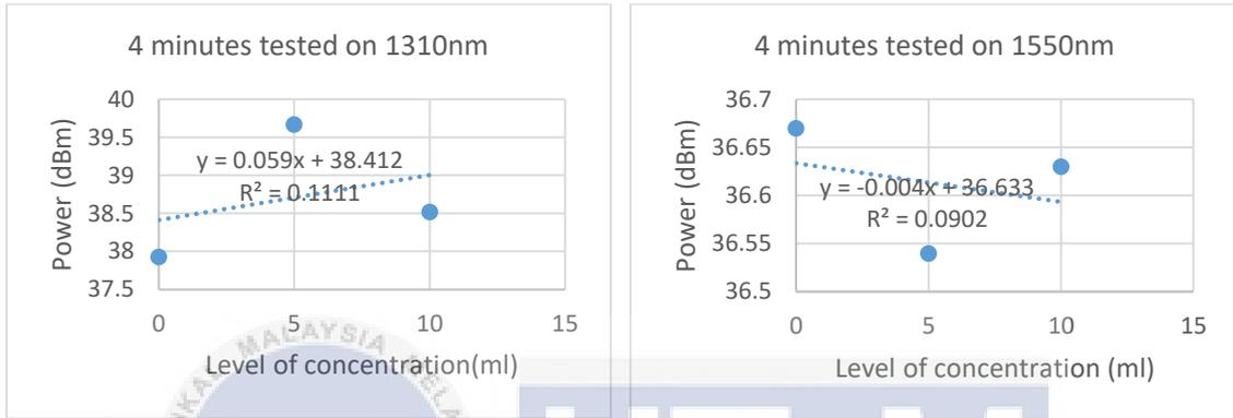
**Figure 4.11 : Microfiber Single Loop Sensor response at 4 minutes**
