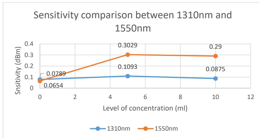
**Figure 4.6 : Comparison of Sensitivity between 1310nm and 1550nm**
