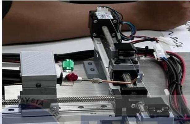
**Figure 3.15 : The process of tapering the fiber optic cable**
