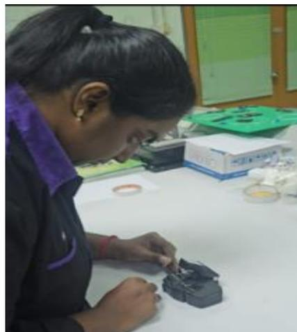
**Figure 3.13 : The process of cleaving the fiber optic cable**
