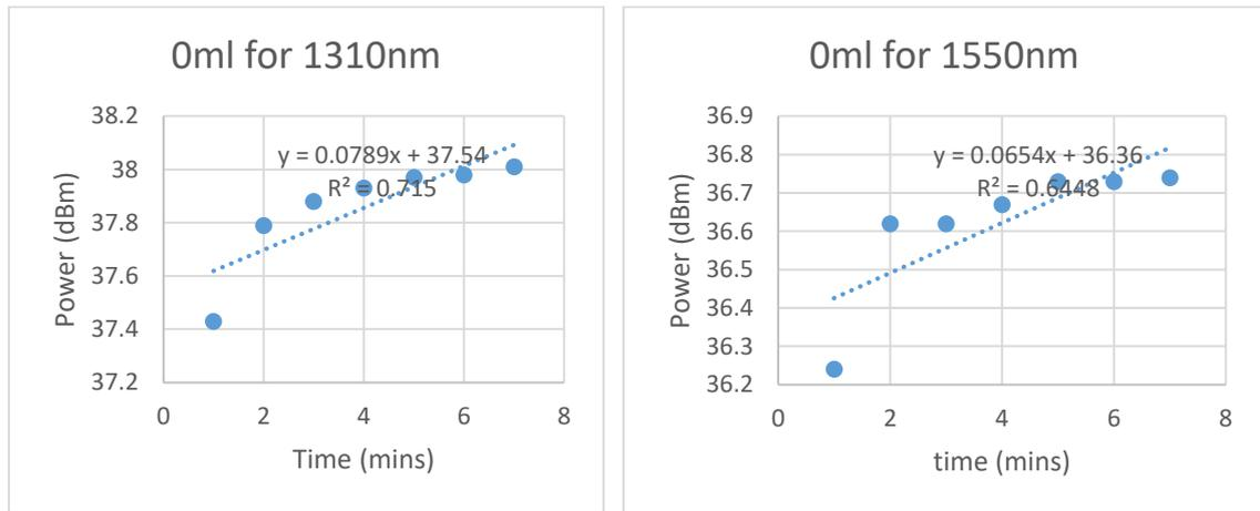
**Figure 4.3 : Microfiber optic single loop sensor response at 0ml**
