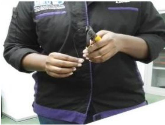
**Figure 3.11 : Fiber optic cable being stripped**
