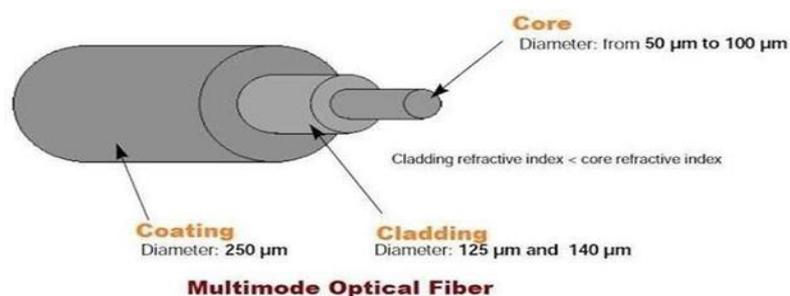
**Figure 2.3 : Multimode Optical fiber**
