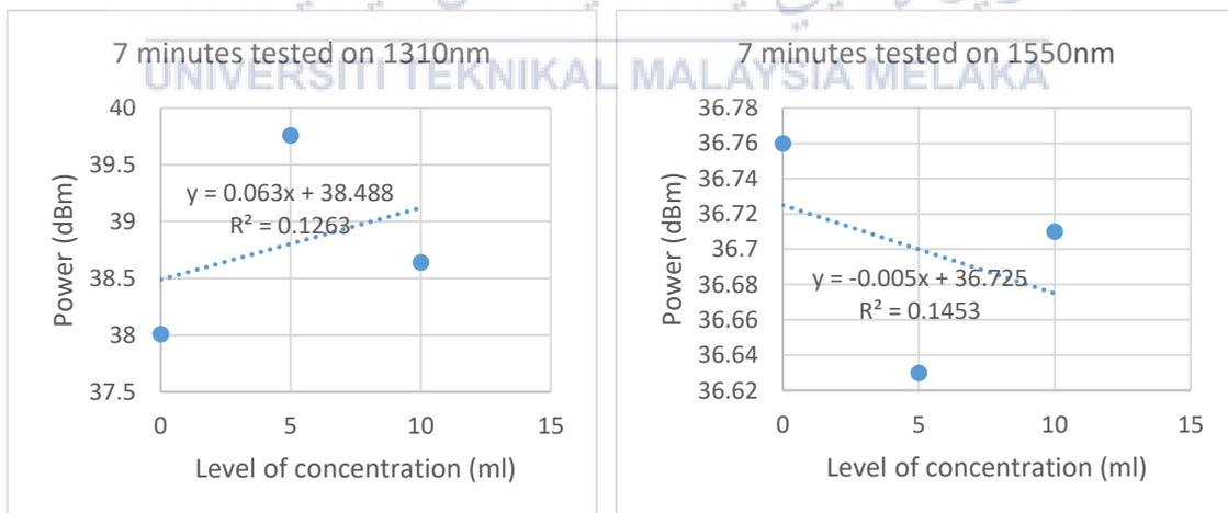
Figure 4.14 : Microfiber Single Loop Sensor response at 7 minutes
