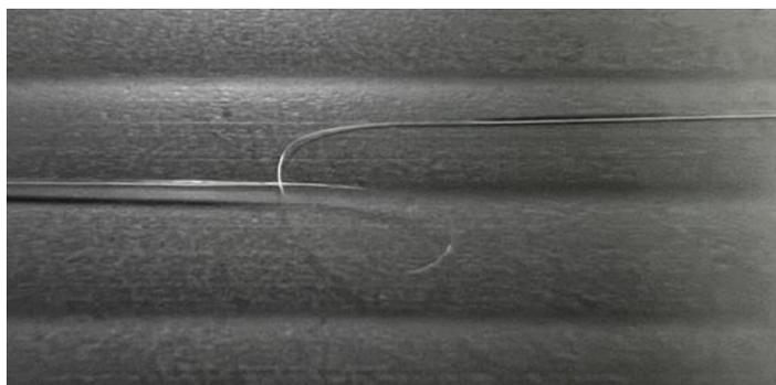
**Figure 3.16 : The process of looping the fibre optic cable**
