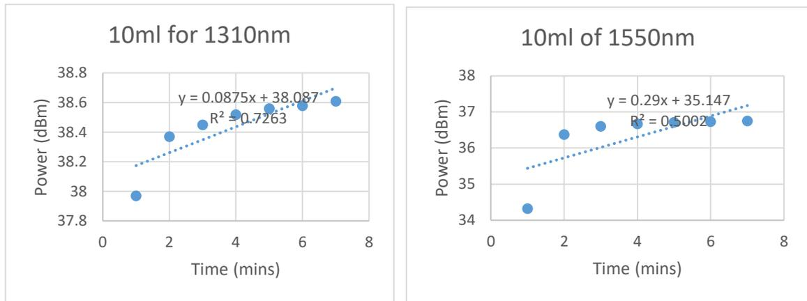
**Figure 4.5 : Microfiber optic single loop sensor response at 10ml**
