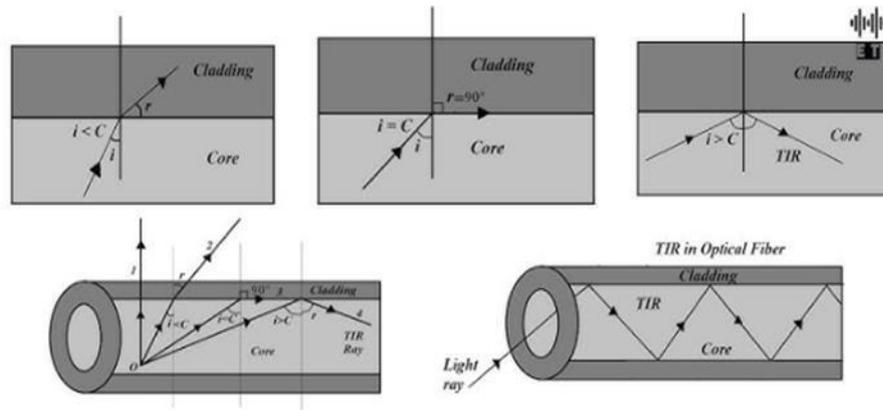
**Figure 2.5 : Light propagation in optical fiber**
