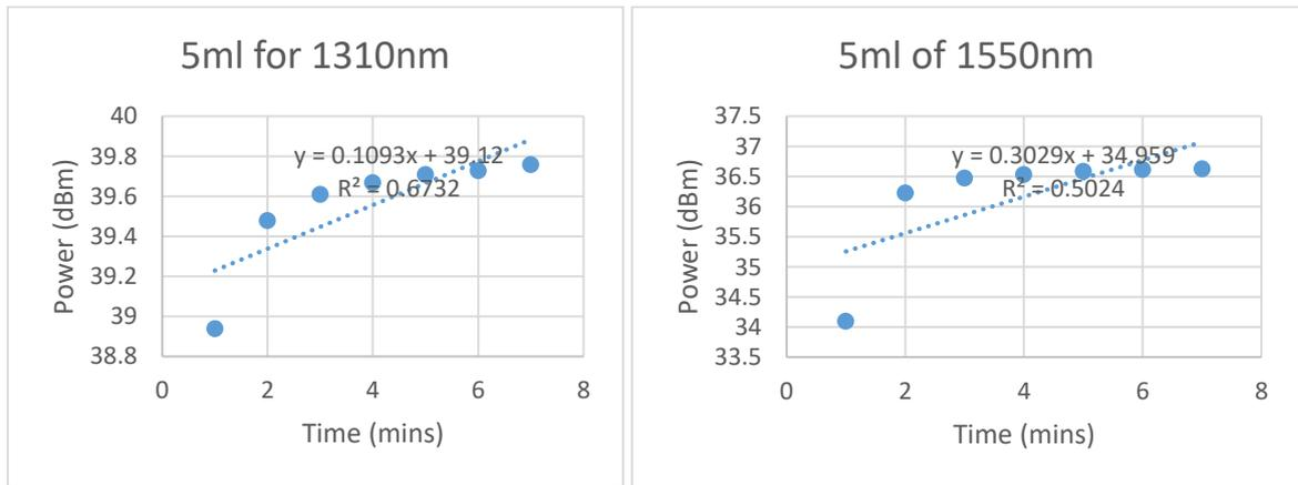
**Figure 4.4 : Microfiber optic single loop sensor response at 5ml**
