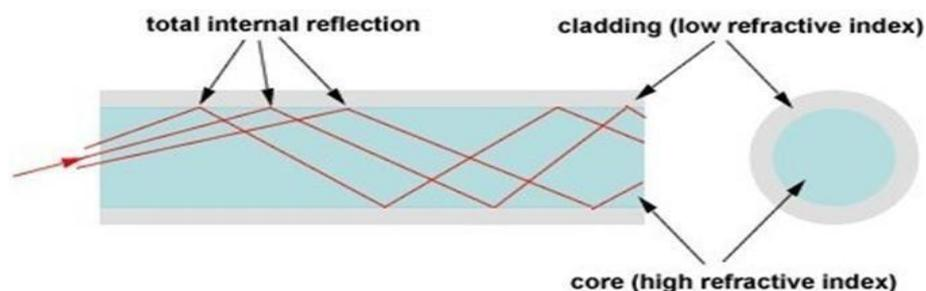
**Figure 2.6 : Total Internal Reflection**
