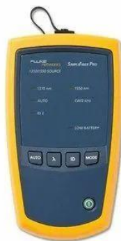
Figure 18.10 Optical Power Meter
