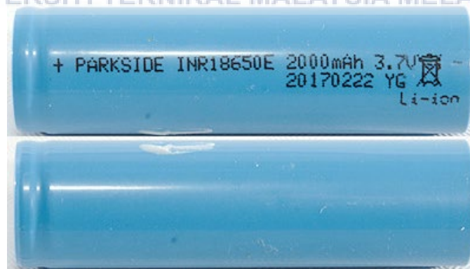
Figure 3.9 INR185650 2000mAh 3.7 7.4Wh Battery[47]
