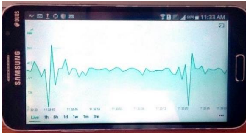
Figure 2.1 ECG output signal on Blynk application [12]
