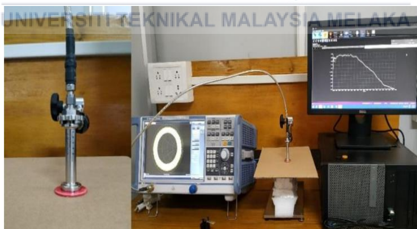
Figure 2.21 Representation of measurement set-up to measure the dielectric properties of the button
