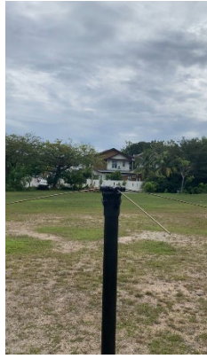
Figure 4.5 : Cross-Dipole Antenna on the Field
