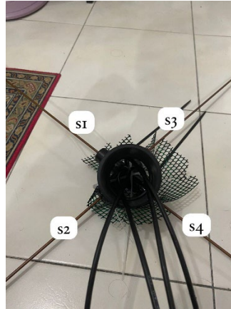
Figure 4.2 : Connection Between Dipole Antenna and Main Coaxial
