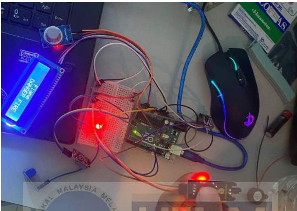
Figure 4.7.2: Hardware of Fire within Smoke
