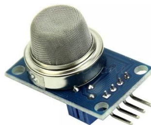
Figure 3.5.5: Structure of smoke sensor (MQ2 sensor)
