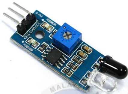
Figure 3.5.4: Structure of Flame Sensor (IR sensor)
