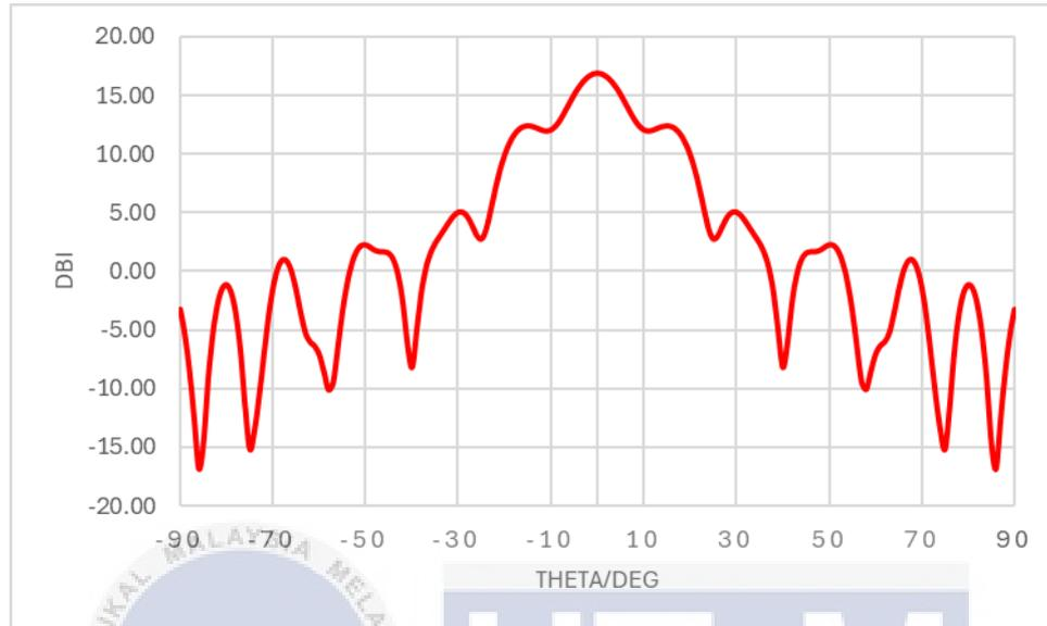
Figure 4.30 Cartesian graph of Farfield gain for 28GHz
