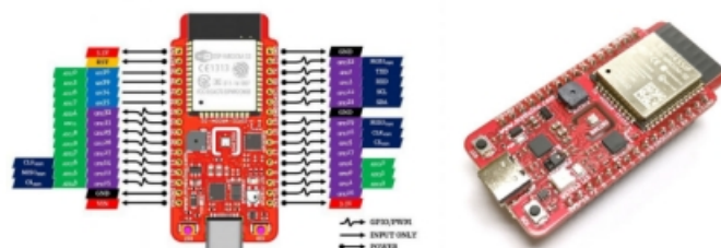
Figure 3.7 Pinout of Hibiscus ESP32
