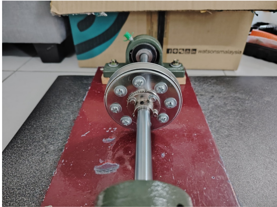
Figure 3.16 Balanced load condition of the testbed
