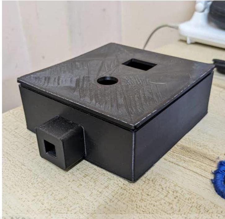
**Figure 3.5: The fabricated prototype's casing using 3D printing method**
