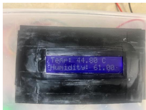
Figure 4.12 : Temperature and Humidity in Solar Still
