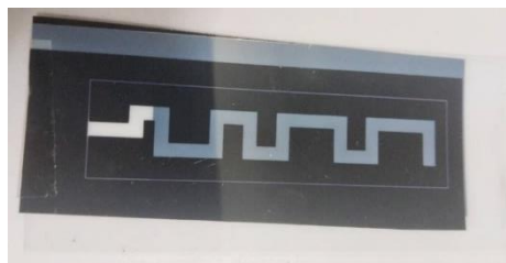
Figure 3.10: Printed MLA design on Transfer Film
