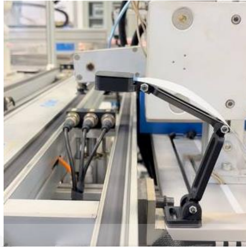
Figure 3.8: Raspberry Pi Camera Module 3 installed on the FMS 200.
