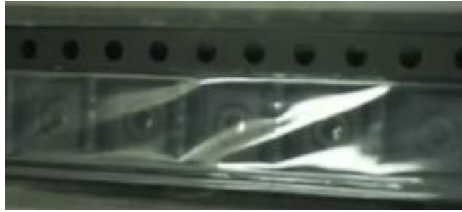
Figure 3.4: Cover tape position away from sprocket hole.
