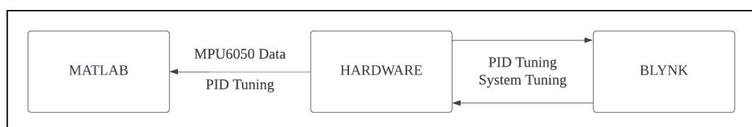
Figure 3.19: Block Diagram for Hardware and Software Integration.
